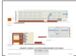
Left: Elevation of West Wall with change to Oyster/Colonial Red Metal Wall Panels. Right: Elevation of East Façade with change to Brick at Construction Yard wall.
